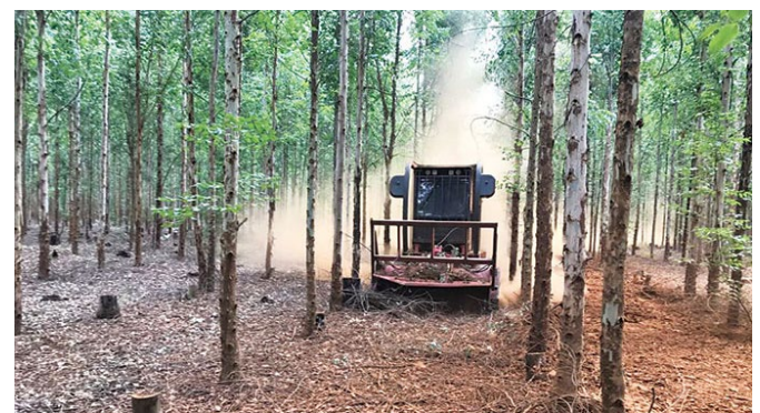
Figure 14: Mulcher working between eucalyptus tree rows
