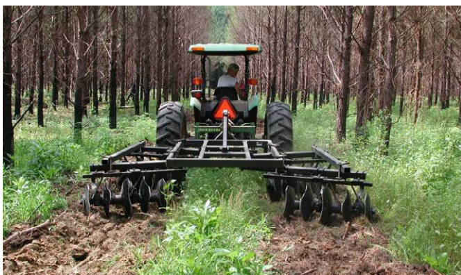
Figure 7: Disking of an internal fire belt
