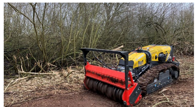
Figure 13: Mulcher incorporating woody material with the soil ( www.prinoth.com/en/vegetation-management )
